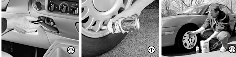
Easy as 1-2-3: 1. Plug in the cord, 2. Install the sealant, 3. Inflate the tire!
