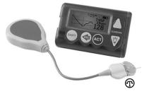
The Guardian REAL-Time System glucose sensor is a tiny electrode inserted under the skin that measures glucose levels, providing patients with better protection against frequent blood-sugar highs and lows.
