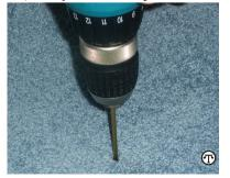
**Step two:** Place your weight around the fixture and drive the scored screw down as far as the fixture allows it to go.
