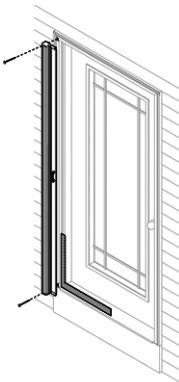
**Step 1 Install the screen housing.**
