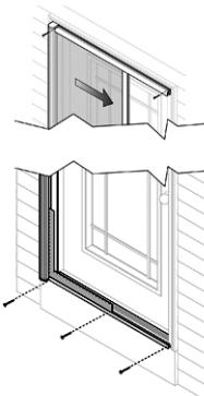
**Step 3 Install tracks and sill plate.**
