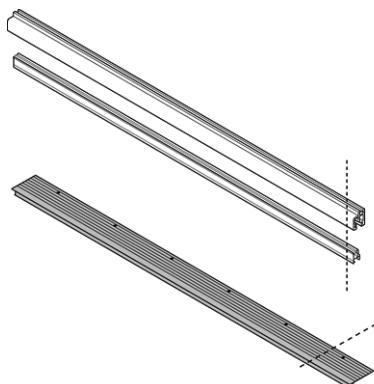
**Step 2 Cut tracks and sill plate to the correct width of your door.**
