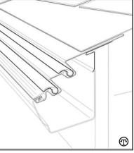
For areas with a high volume of small debris (seed buds, pine needles) the Small Debris Insert is recommended.
