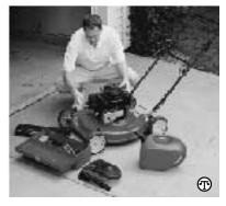
filter. If the engine requires a foam-type filter, remove the sponge from the filter assembly, soak it in a pan of warm water and squeeze it dry. Then apply a few drops of clean oil into the sponge and place it back in the filter assembly.
