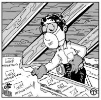
Insulation is ranked by R-value. The higher the R-value, the better your walls and roof will resist the transfer of heat when it's installed.
