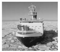
The bow does not cut through the ice like a knife. The icebreaker pushes itself on top of the ice and the ice breaks under its weight.
