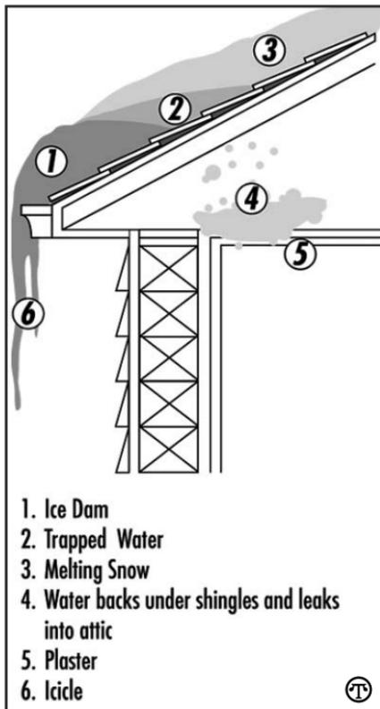
**Melting snow trickles to the roof's edge, creating an ice dam, which in turn creates internal leaks.**
