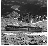
A special motor converts a descending locomotive's energy into electricity.
