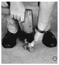
Step 2: DRIVE THE SCREW Place your weight around the fixture and drive the scored screw down as far as the fixture will allow it to go.
