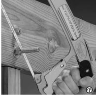
Flush Cuts—A flexible blade can be switched from the 90° configuration to a 45° one to allow for hard-to-reach flush cuts.
