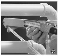
Tight Cuts—The front section of the frame flips up and out of the way of the blade so the saw can be used in tight spaces.
