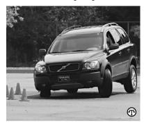
Electronic Stability Control (ESC) builds on ABS and TCS and is a stability enhancement system designed to electronically detect and automatically assist drivers in critical driving situations. ESC compares the driver's intended course with the vehicle's actual course and compensates for any differences. As one auto expert says, "It's the greatest feature in your car you'll never know sayed your life."
