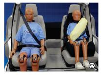
Inflated seat belts distribute crash force energy across up to five times more of the rider's torso than a traditional belt, expanding the range of protection and reducing risk of injury, while providing additional head and neck support.
