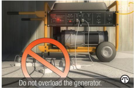
**Plug appliances directly into the generator or use a heavy-duty, outdoor-rated extension cord. And make sure not to overload the generator.**
